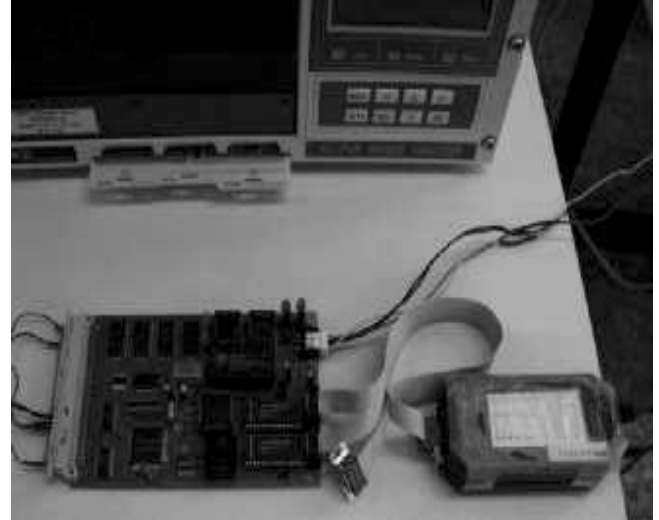
Fig. 2. Local unit micro-controller based prototype, GSM phone, and SO2 sensor.
