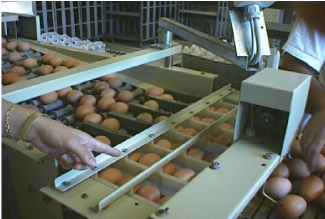
Figure 1. Mechanized conveyor belt with six channels, index finger points to the best location to insert a vision system endowed of six aligned color cameras.
