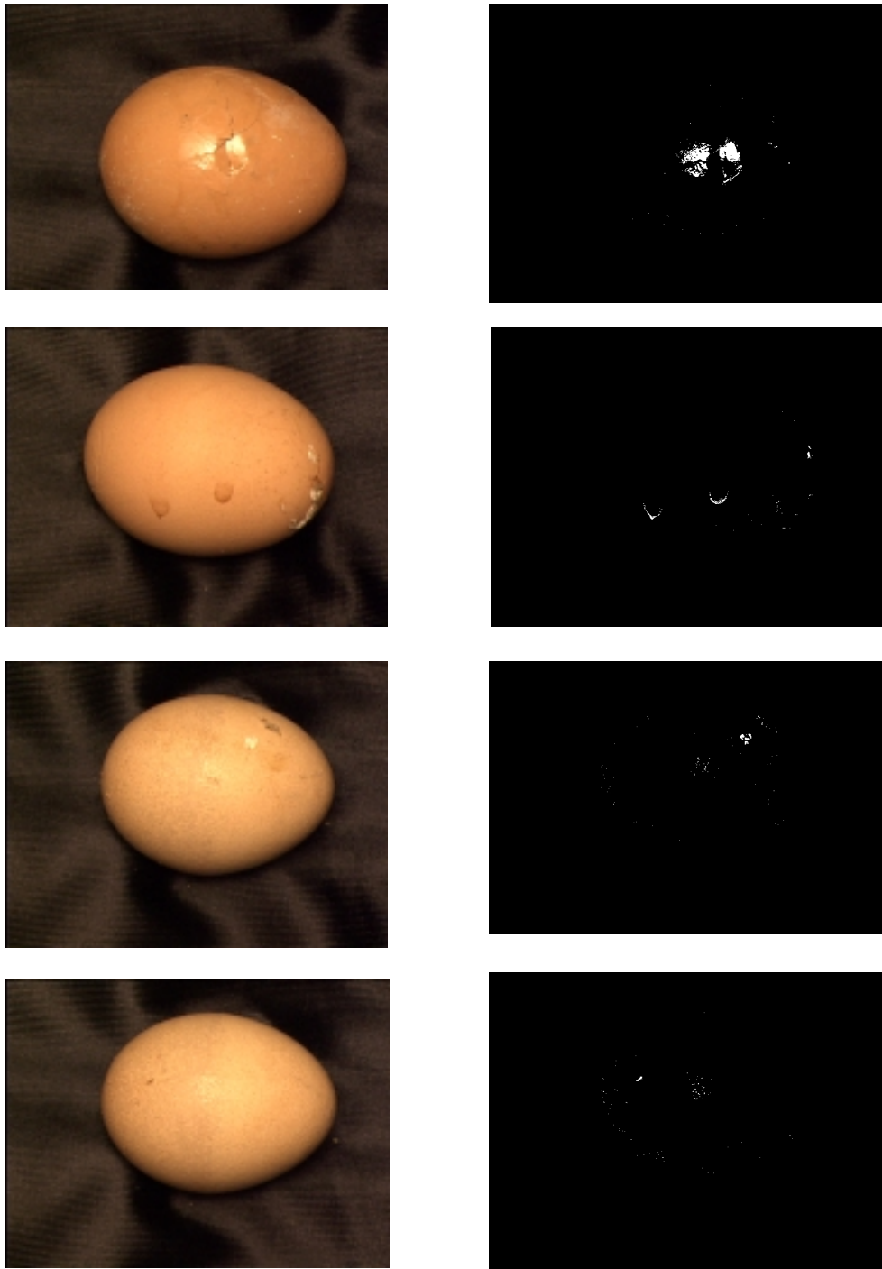
Figure 2: Examples of different types of defects: Original colour images and Binary images.
