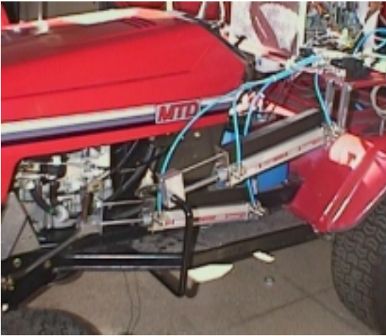
Figure 2: Axle, piston, cylinder and electrovalve detail
